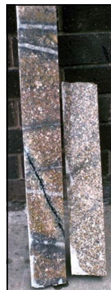
Figure 12 (Right). Cores of mineralised and unmineralised granite from beneath the kaolinised zone at Hemerdon.
